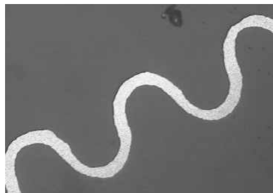
Fig. 3. Image of polysilicon fiber after lift-off, 1 \mu\text{m} thick polysilicon, 35 \mu\text{m} wide.
